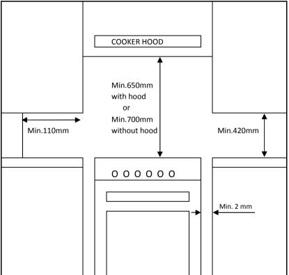
This cooker may be fitted flush to the base units. Leave a gap of approximately 2mm minimum from any adjacent cupboard or appliance. Any adjacent surface must be heat resistant to  $50^{\circ}$ C and if it is higher than the appliance it must be a minimum of 110mm away from the appliance. Any such adjacent cupboard less than 110mm away horizontally, must be at least 420mm higher than the hotplate level.
