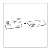
4. Unscrew middle hinge. Then lift lower door and place it on a soft pad to avoid scratching.
