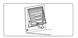
To replace the wire racks, firstly hook the guides back in to the locating holes then push the rack back in to the clips (a).
