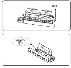
Remove the injectors using a 7mm spanner and replace the injector with the ones from the spare set. Make sure you use corresponding diameters suitable to the type of gas that is going to be used, according to the information chart (which is also supplied in the gas conversion kit).
