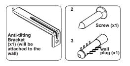
The document bag contains an anti-tilting kit. Loosely attach the anti-tilting bracket (1) to the wall using the screw (2) and wall plug (3), following the measurements shown in the figure and table below. Adjust the height of the antitilting bracket so that it lines up with the slot on the cooker and tighten the screw. Push the appliance towards the wall making sure that the anti-tilting bracket is inserted into the slot on the rear of the appliance.
