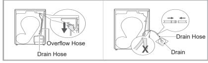
Carefully pull down and remove the drain hose from the tank housing (making sure to remove the drain hose and not the overflow hose). Connect the drain hose extension and securely place the end of the hose in a sink, sink trap or separate stand pipe (be careful not to bend the external drain hose).
