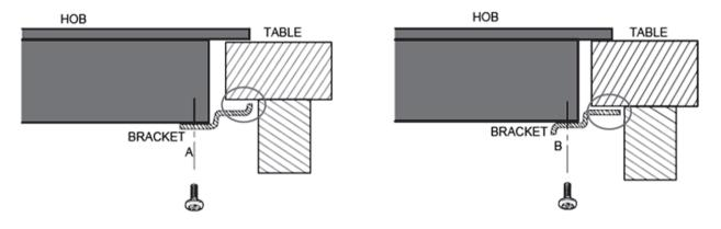
Under any circumstances, the brackets cannot touch with the inner surfaces of the worktop after installation (see picture).
