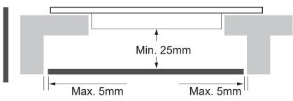
There are ventilation holes around outside of the hob. YOU MUST ensure these holes are not blocked by the worktop when you put the hob into position.
